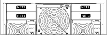
Figure 40: Slots for the LAN I/O blades
